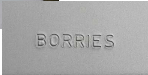
Test marking with 3 mm font height on eloxadized aluminum
